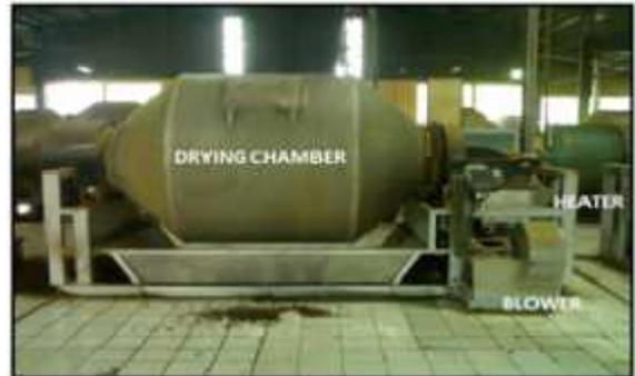
Gambar 1. Photo Alat pengering berputar (*rotary dryer*).
